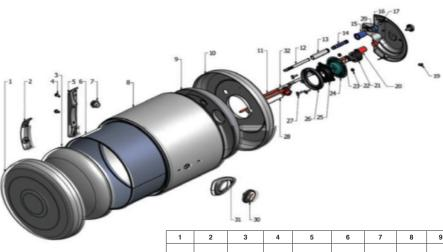
10 11 12 13 16 Spacer Tub (Blue) Outer Upper Cover Inner Upper Dome Outer Hanging ½" Pipes 17 20 21 23 25 26 29 32 Electrical Cover Indicated Lamp 5 Nut's M6\*1.25 Flange Tank Thermometer Frame
