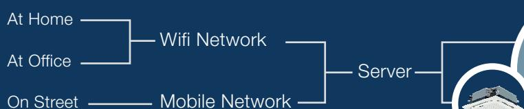
Based on Rheem's cloud web system and with the android system platform a wifi module is provided in the air conditioners to achieve different functions through terminals(mobile phone, iPad and computer) for easy and visualized operation.
