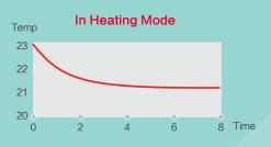
While set on sleep mode, the air conditioner will automatically decrease set temperature 1°C (ST+1°C) 1 hour later, ST+2°C after 1 more hour and keep the same condition after that.
