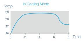
While set on sleep mode, the air conditioner will automatically increase set temperature 1°C (ST+1 °C) 1 hour later, ST+2 °C after 1 more hour and keep the same condition after that .
